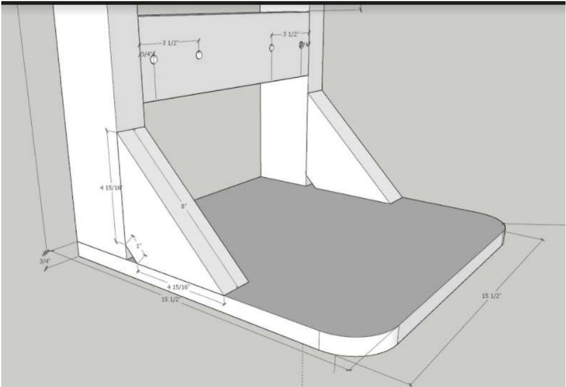
Fig. 4.0 (Measurements for the Base Board and Angle Piece)
