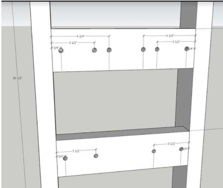
Fig. 5.0 (Measurements for Cross Pieces)
