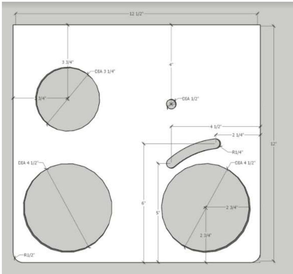
Fig. 3.0(Measurement for the Fan Deck Board)
