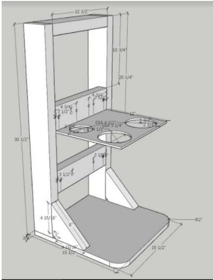
Fig. 2.0(Measurements for the whole frame)
