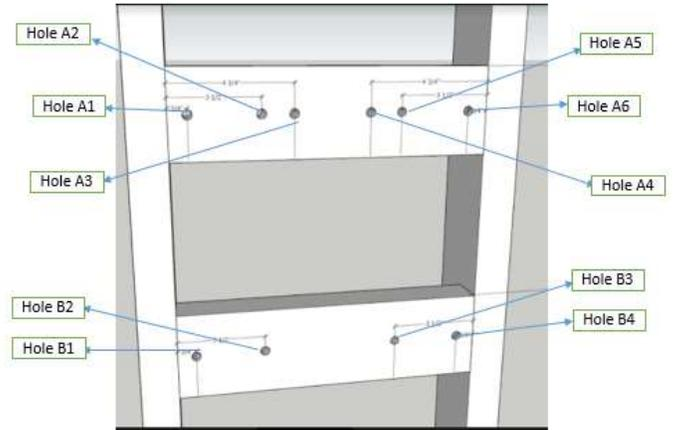
Fig.8.0 (Hole Assignment for Cross Pieces)
