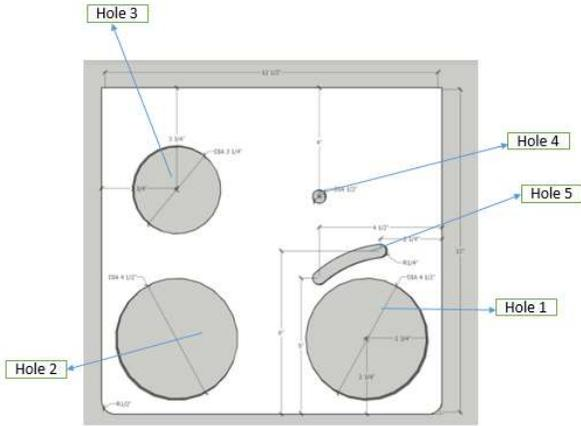
Fig.7.0 (Hole Assignment for Fan Deck Board)
